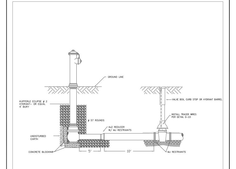
HYDRANTS SHALL BE SET IN 4 CUBIC FEET OF CRUSHED STONE TO ALLOW FOR PROPER DRAINAGE OF THE HYDRANT. RECOMMENDATIONS OF THE AWWA SHOULD BE FOLLOWED WHEN INSTALLING THE HYDRANTS.
