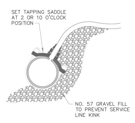
NOTE: SADDLES SHALL BE MODEL FORD S70 FOR PVC AND FORD S90 FOR C900. TAP SET AT 12 O'CLOCK FOR ALL AIR RELEASE APPLICATIONS.
